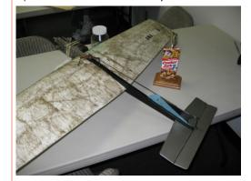
**Larry Renger** – He showed the horizontal tail surfaces of a Baby Clown that were hinged using strips of Polyspan. By the time the stab and elevator were covered with silkspan, the hinges disappear. They remain very flexible!
